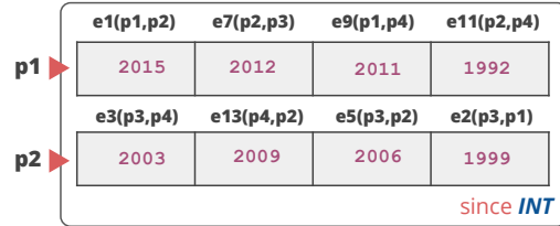
Figure 4: Single-indexed property pages for since property of FOLLOWS edges in the example graph. k = 2 .
